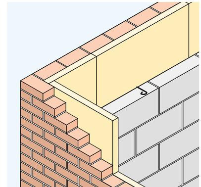
Figure 8 Batts close butted at corners
