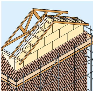
Figure 9 Installation of Batts in gable end wall
